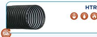
TEMPERATURE RANGE: -40° F to 225° F CONSTRUCTION: Polypropylene reinforced with a polypropylene rod helix STANDARD COLOR: Black STANDARD LENGTHS: 25' & 50' SIZE RANGE: 1.5", 2", 2.5", 3", 4"
