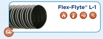
TEMPERATURE RANGE: -65° F to 300° F CONSTRUCTION: Two-ply neoprene coated fiberglass STANDARD COLOR: Black STANDARD LENGTHS: 12' & 25' SIZE RANGE: 2", 2.5", 3", 4", 5", 6", 8"
