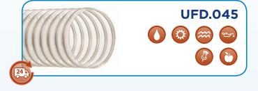
TEMPERATURE RANGE: -65° F to 200° F CONSTRUCTION: Heavy walled polyurethane reinforced with a wire helix STANDARD COLOR: Clear STANDARD LENGTHS: 25' & 50' SIZE RANGE: 4", 6", 8"
