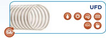
TEMPERATURE RANGE: -65° F to 200° F CONSTRUCTION: Polyurethane reinforced with a wire helix STANDARD COLORS: Clear or Black STANDARD LENGTHS: 25' & 50' SIZE RANGE: 3", 4", 6", 8", 10"
