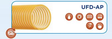
TEMPERATURE RANGE: -40° F to 200° F CONSTRUCTION: All polyurethane hose reinforced with an ABS helix STANDARD COLOR: Clear with a safety yellow helix STANDARD LENGTHS: 25' & 50' SIZE RANGE: 2", 3", 4", 6", 8"
